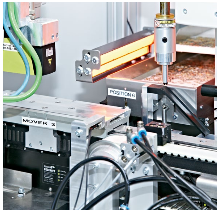
The decoupling of transfer system and process stations is particularly important in the assembly of small parts.
