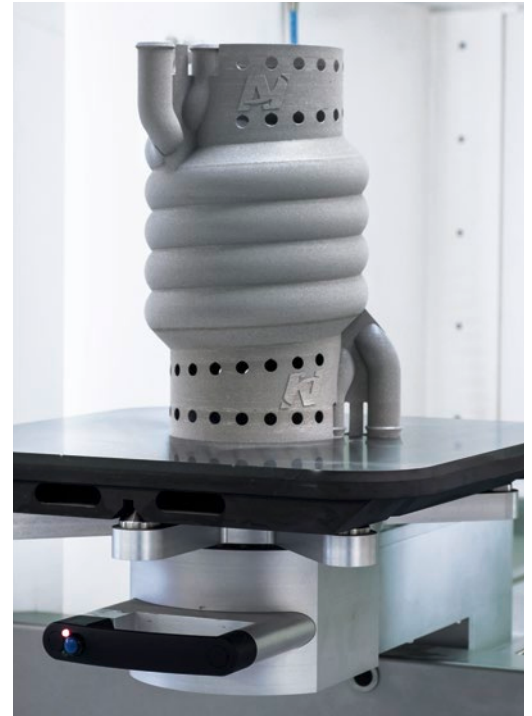
A heat exchanger produced with the 3D printing method
