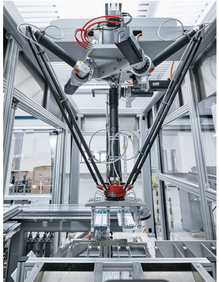
The two HSPP systems at the start and end of the labeling and grouping unit employ dynamic Beckhoff drive technology and are controlled together with the XTS via a single C6930 control cabinet PC.
