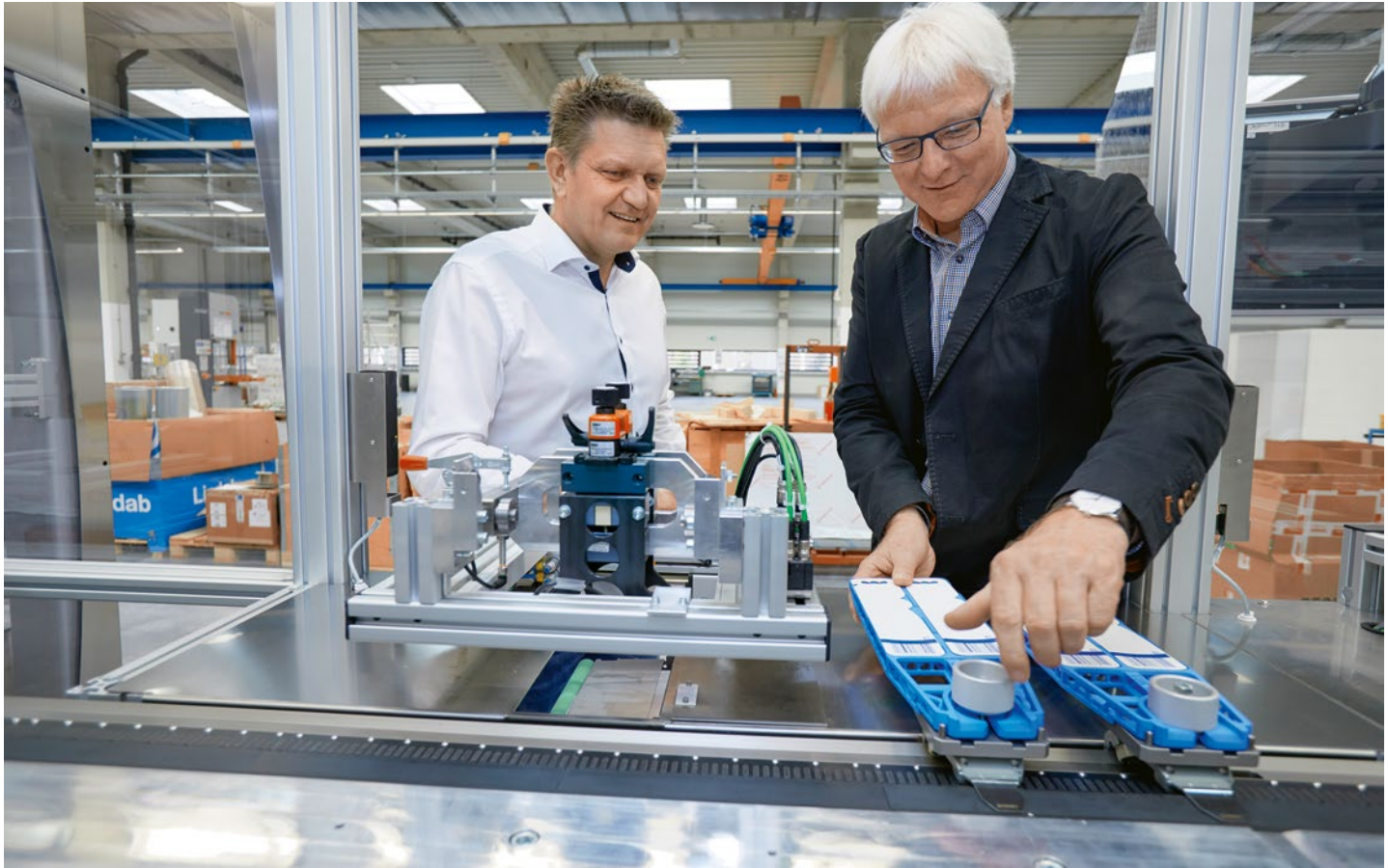
Jürgen Welker (right) of Koch Pac-Systeme shows Frank Würthner of Beckhoff how easy it is to switch out the blister carriers for rapid product changeovers.
